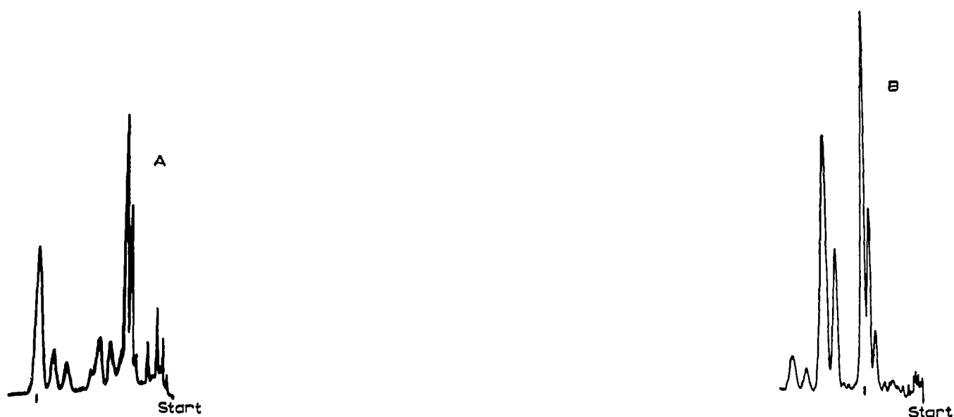
Fig. 2. (A) Reduction products from 5 \mu g 16 \alpha -hydroxydehydroepiandrosterone, catalyst temperature 200 ^{\circ} , chromatographed on an NGA coated column at 150 ^{\circ} ; attenuation \times 100. The retention time of 5 \alpha -androstane is indicated by a vertical line. (B) Reduction products from 10 \mu g cortisol, catalyst temperature 190 ^{\circ} , chromatographed on an SE-30 coated column at 160 ^{\circ} ; attenuation \times 100. The retention time of 5 \alpha -androstane is indicated by a vertical line.
